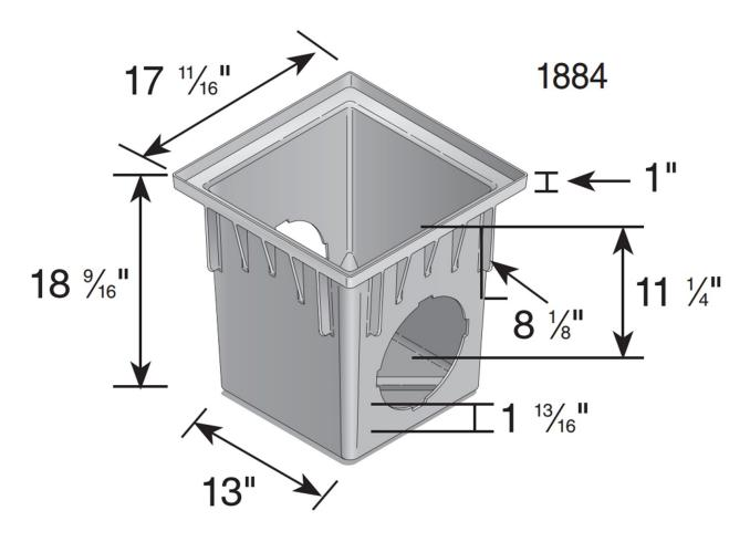
Material: UV Protected High Density Polyethylene (HDPE)
